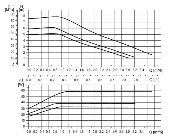
UPM3 K FLEX AS 25-75 180 electrical parameters, 1 x 230 V, 50/60 Hz
