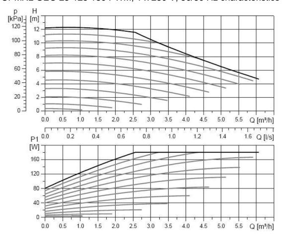
UPMXL GEO 25-125 180 PWM electrical parameters, 1 x 230 V, 50/60 Hz
